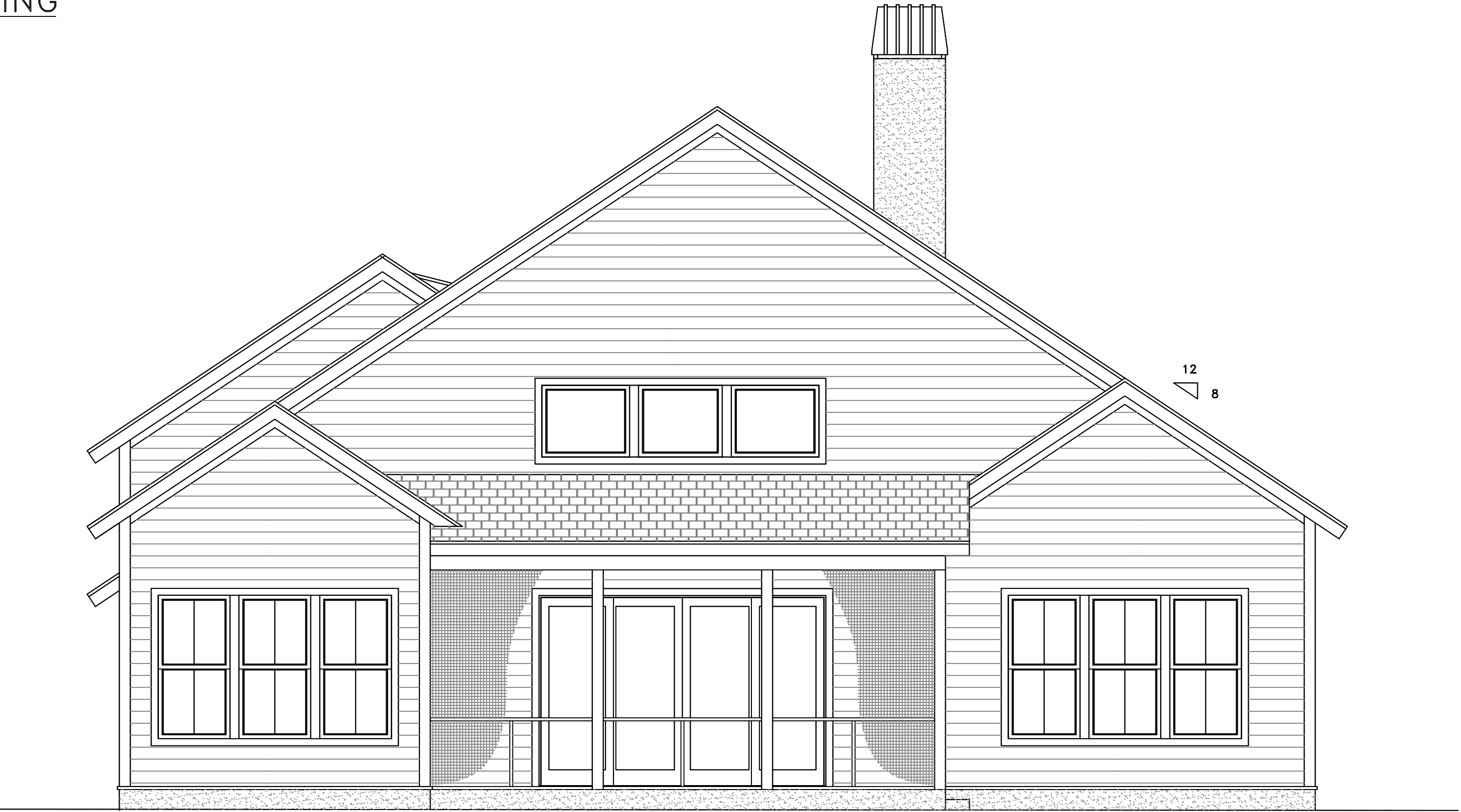
REAR ELEVATION W/SCREENED PORCH SCALE: 1/4" = 1'-0"
